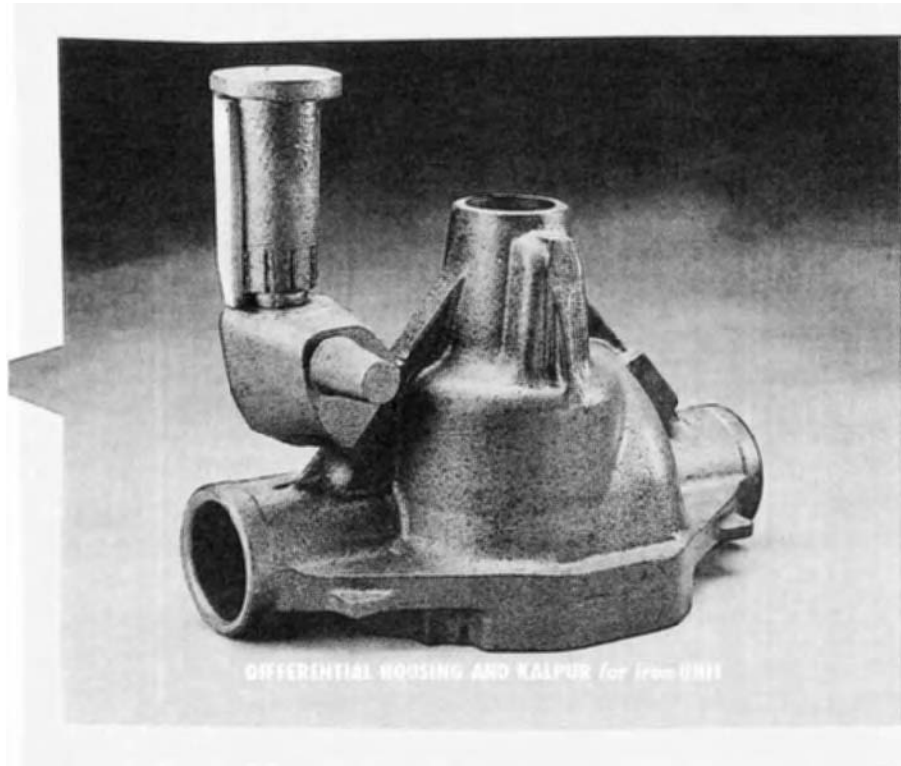
Figure 17.26 Ductile iron differential housing made on a DISAMATIC 2070 moulding machine with a KALPUR unit.
