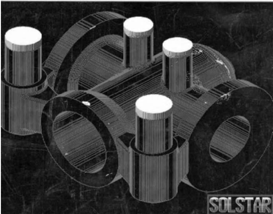
Figure 20.3 An 'X-ray' plot showing predicted shrinkage cavities. (This figure is reproduced in colour in plate section.)
