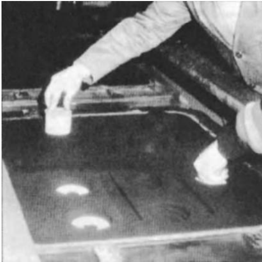
Figure 19.11 The KALSERT system in operation. KALMINEX sleeves being inserted into green sand moulds on an automatic moulding line.
