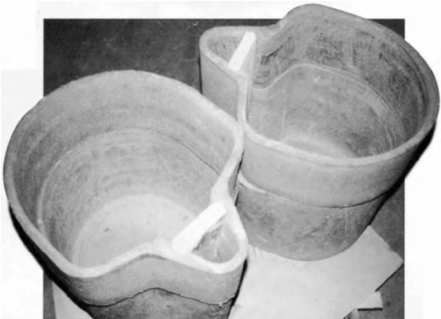
Figure 11.3 1100 kg capacity teapot KALTEK ladle.
