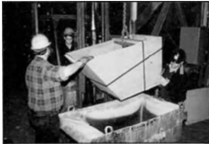
Figure 11.5 Lowering the pre-assembled KALTEK boards into the DISAMATIC automatic pouring box.
